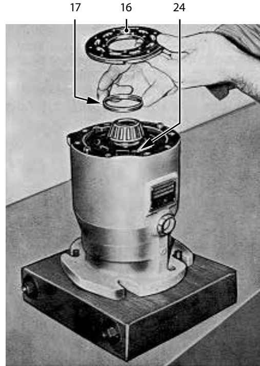
Install the pilot ring and the locating pin in the cylinder block.
